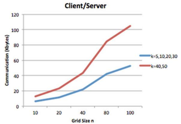
Fig. 6. Performance of our basic protocol for communication (where  $m = 10$ ).
