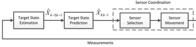
Fig. 1. Framework of target tracking and sensor coordination.
