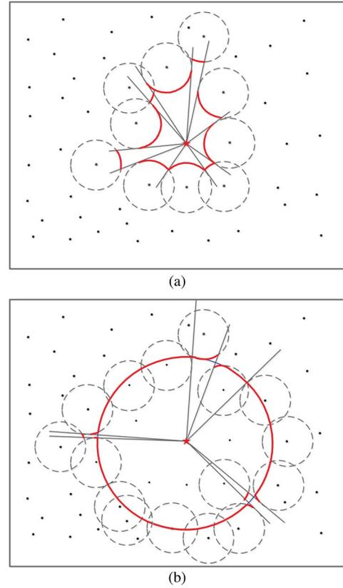
Fig. 4. Profiles of sensor exclusion under two cases of MN. (a)  $2\sigma_\omega^2 < (1 + \mu_\omega)^2$ . (b)  $2\sigma_\omega^2 > (1 + \mu_\omega)^2$ .
