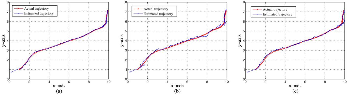
Fig. 5. Comparison between the true trajectory of the target and the estimated trajectories by three different strategies. (a) Proposed strategy. (b) Strategy of random mobile sensor selection. (c) Strategy of optimal static sensor selection.
