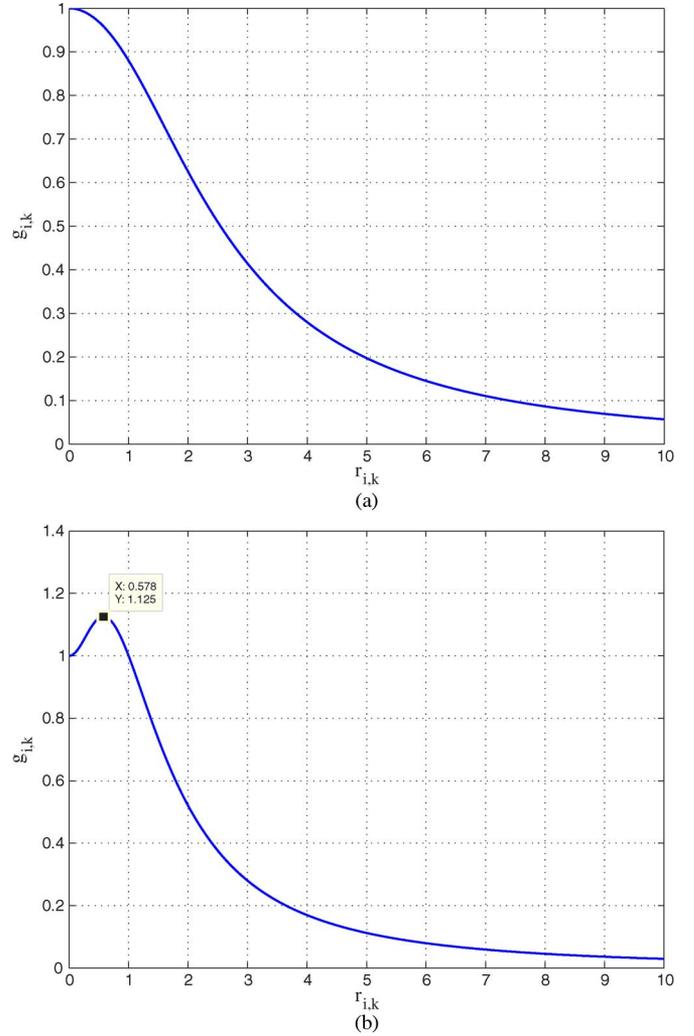
Fig. 2. Profiles of  $g_{i,k}$  under two cases. Let the AN be  $v_{i,k} \sim N(0, 1)$  and the MN satisfy (a)  $2\sigma_\omega^2 < (1 + \mu_\omega)^2$  and (b)  $2\sigma_\omega^2 > (1 + \mu_\omega)^2$ .
