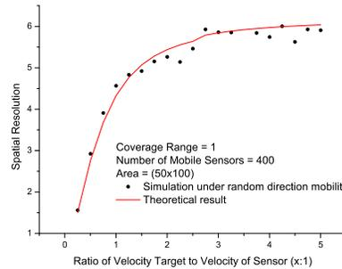
Fig. 9. The spatial resolution against ratio of target speed to sensor speed.
