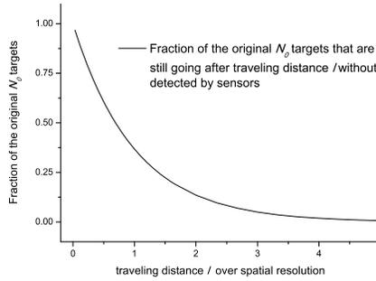
Fig. 6. Fraction of the original  $N_0$  targets that are still going after traveling distance  $l$  without detected by sensors
