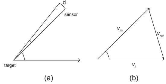
Fig. 4. (a)The speed of the moving target relative to one of mobile sensors varies only with the angle between their respective directions of motion; (b)The relative speed  $v_{rel}$ .
