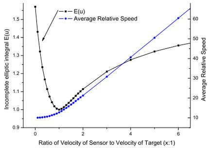
Fig. 5. Incomplete elliptic integral function and average relative speed  $\bar{v}_{rel}$  against ratio of sensor speed to target speed.
