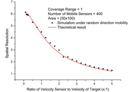
Fig. 10. The spatial resolution against ratio of sensor speed to target speed.
