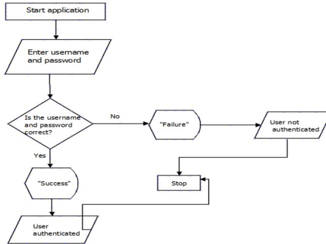
Figure 3 : Flowchart for user authentication process
